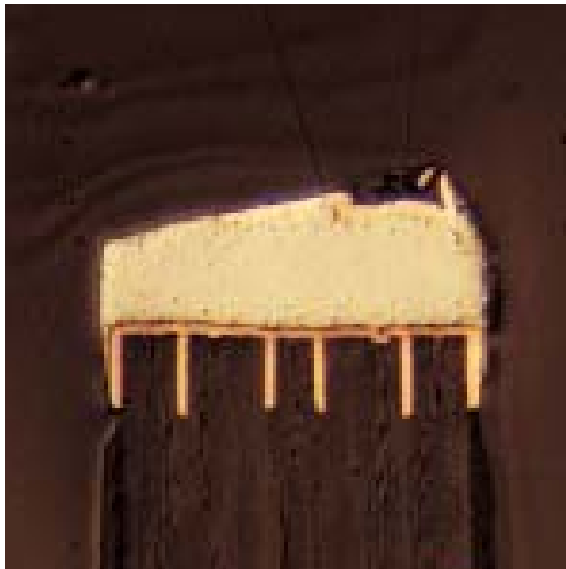
Multi-layer circuit board, crack resulting in poor contact. Original image scales 37:1 and 600:1
